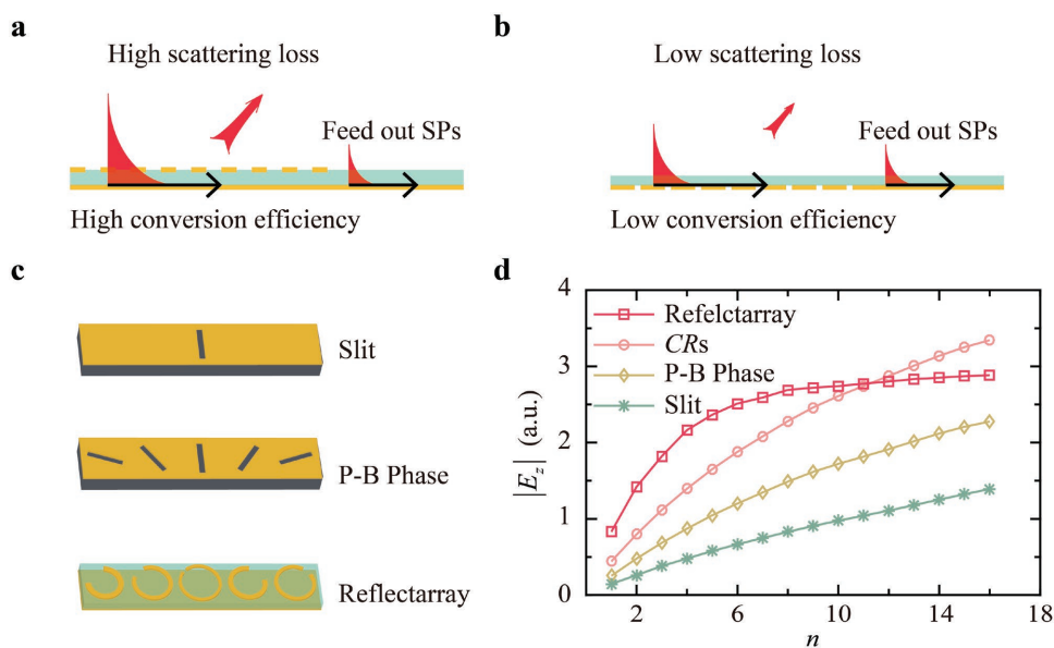
Figure 6. Comparison of different SP excitations. a) and b) Coupling and propagating characters of reflection-type and single-layer SP metacouplers, respectively. c) Schematics of normal slit, P–B phase-based slit array, and reflection-type C-ring-based super units, respectively. Here the width and length of slits are 10 and 70 \mu\text{m} , respectively; the orientation angle difference of adjacent slits in P–B phase-based slit array is 36^\circ ; the geometrical parameters of C-ring resonators are r = 32, 34, 36, 33, 35 \mu\text{m} , \alpha = 95^\circ, 47^\circ, 15^\circ, 70^\circ, 30^\circ , \beta = 135^\circ, 135^\circ, 135^\circ, 45^\circ, 45^\circ , and w = 9, 7, 5, 8, 6 \mu\text{m} , respectively; the thickness of dielectric spacer is 30 \mu\text{m} . d) Simulated E_z -field amplitudes as a function of super unit number n .
